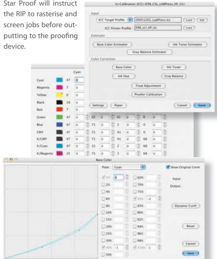
New ICS3 Calibration System enables users to import press and proofer ICC profiles to achieve accurate results easily
