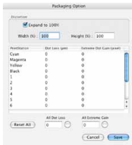
Packaging options for dot distortion, lost dots and extreme dot gain adjustment
